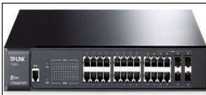
Switch TP-Link TL-SG3424
