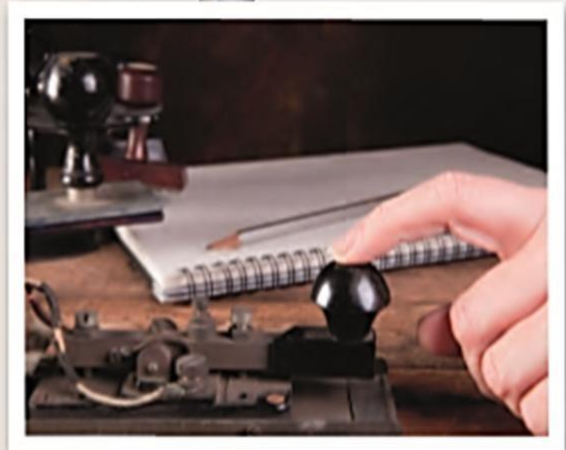
Above A device used to send Morse code.
