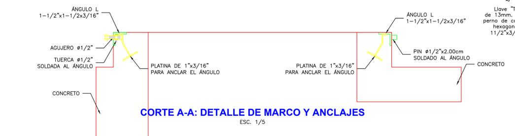
CORTE A-A: DETALLE DE MARCO Y ANCLAJES
