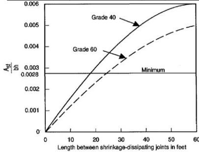
Figure 3 – Minimum temperature and shrinkage reinforcement ratio (ACI 350)
