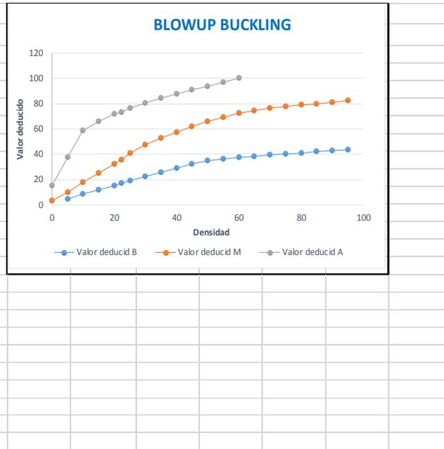
Figura 54; Falla 21 Blowup – Buckling
